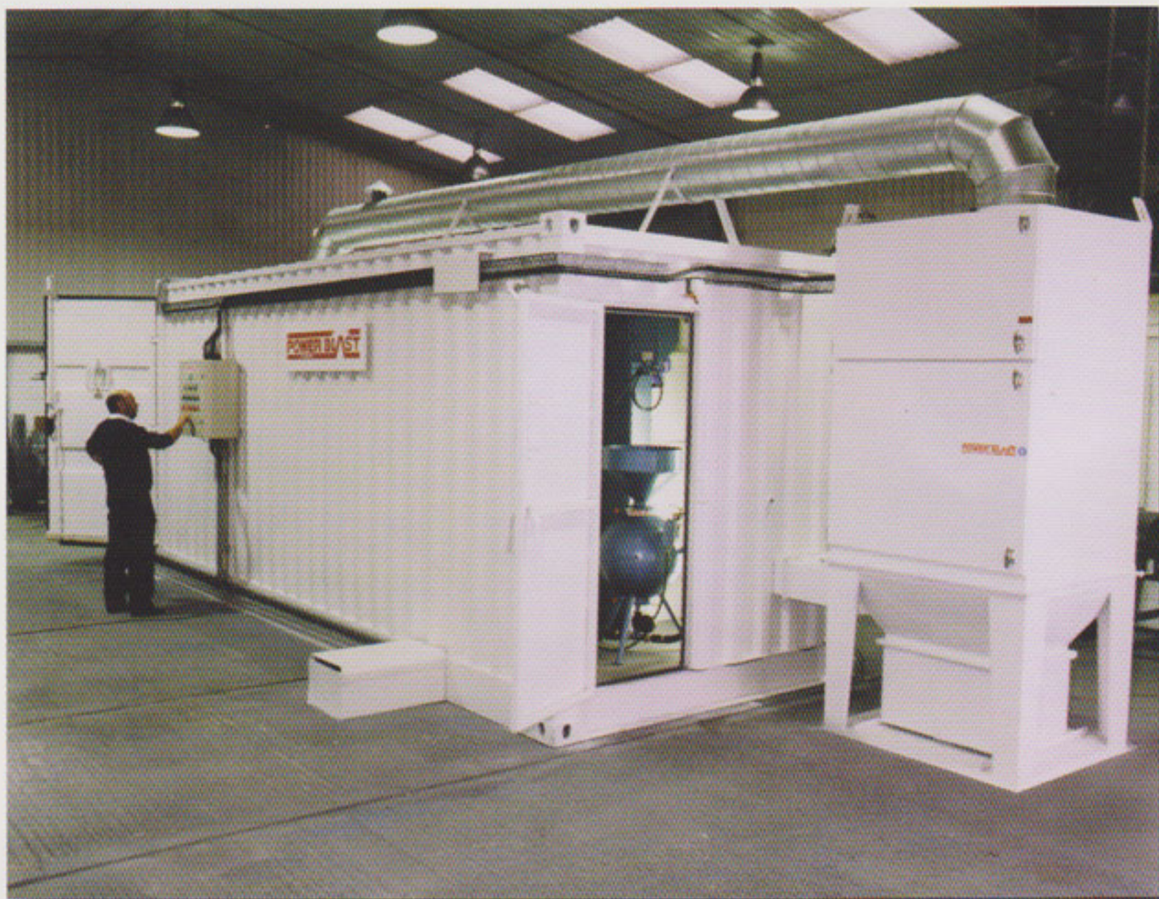
Standard 20' unit with automatic abrasive recovery and external dust collector
